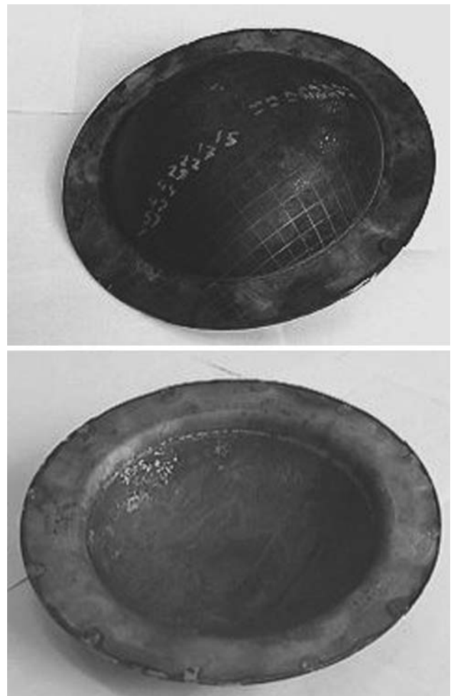
Fig. 4 Workpiece shaped superplastically
